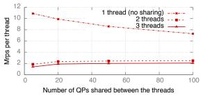
Figure 3: Per-thread READ throughput with QP sharing (CIB)
