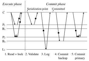
**Figure 6:** FaSST's transaction protocol with tolerance for one node failure.  $P_1$  and  $P_2$  are primaries and  $B_1$  and  $B_2$  are their backups. *C* is the transaction coordinator, whose log replica is  $L_1$ . The solid boxes denote messages containing application-level objects. The transaction reads one key from  $P_1$  and  $P_2$ , and updates the key on  $P_2$ .
