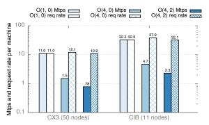
**Figure 7:** Object store performance. The solid and patterned bars show transaction throughput and RPC request rate, respectively. The Y axis is in log scale.
