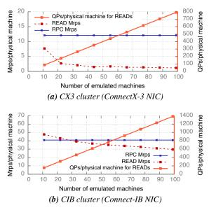
Figure 2: Comparison of FaSST RPC and READ throughput, and the number of QPs used for READs with increasing *emulated* cluster size.
